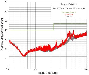
Measured on module with PCB and without external filters at 3m antenna distance
