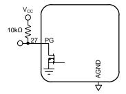
$V_{CC} = V_{IN}$  or other supply voltage below 6V
